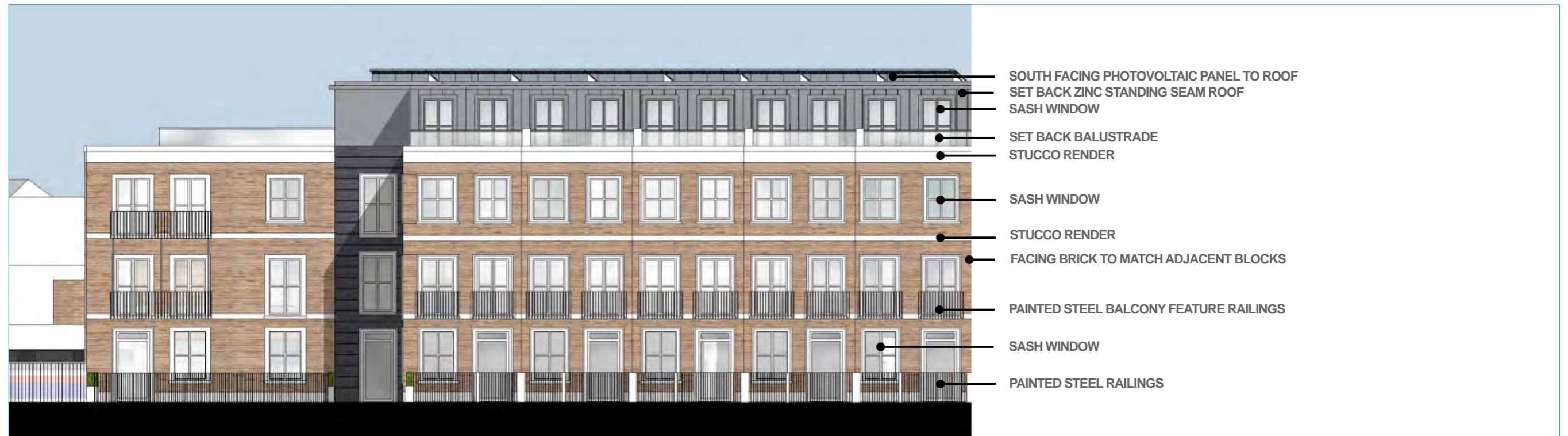
Figure 4.23 Cole Park Road Elevation (Block C)
