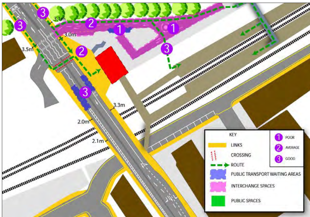
Figure 3: Result of Review of the Existing Catchment Area on a Match Day
