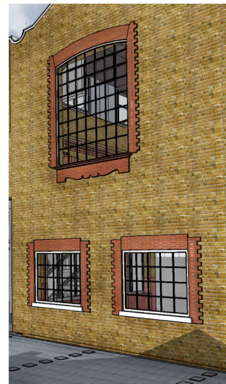
Window reveal quins and arches to new windows
