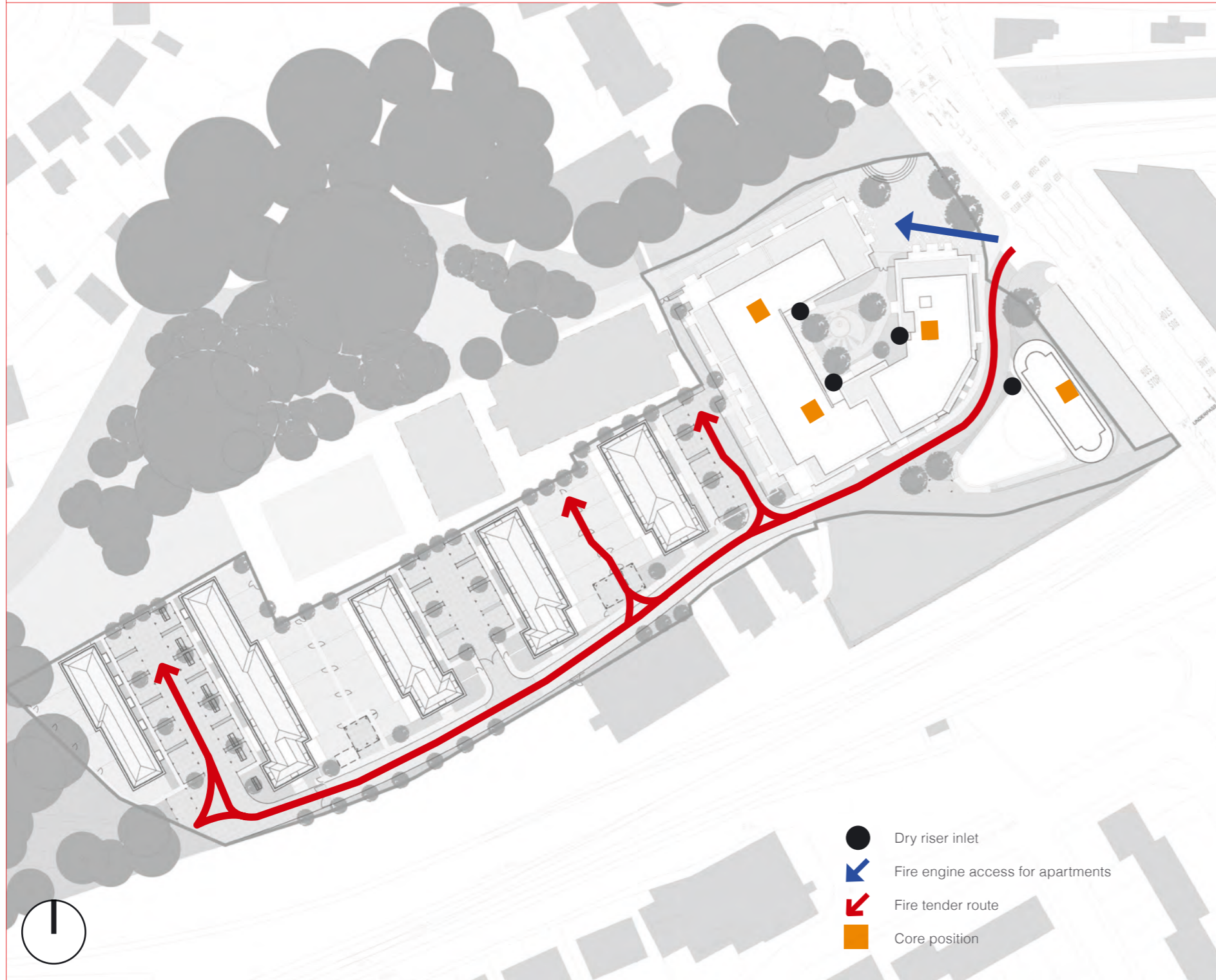
Fire & Emergency Access
