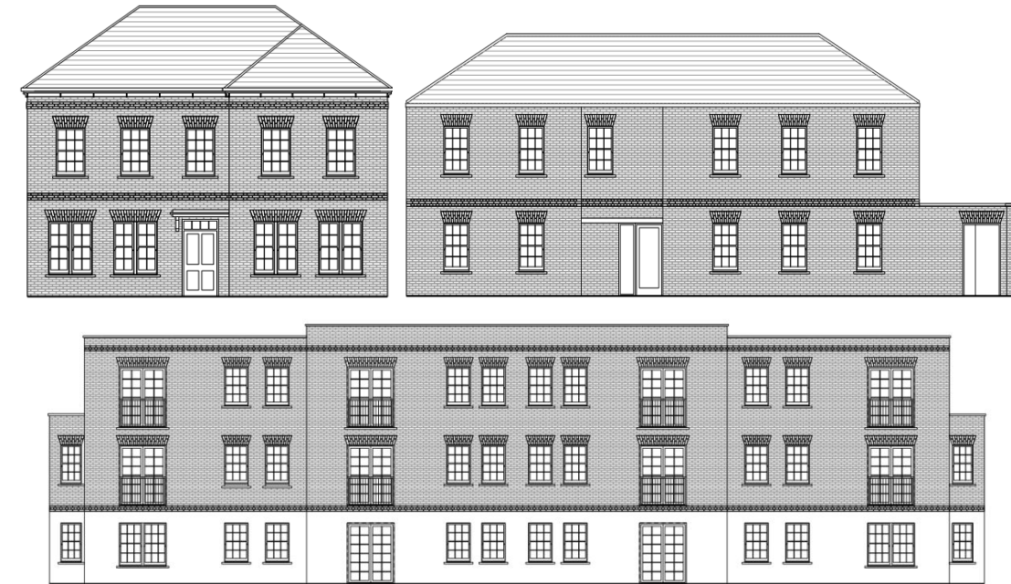
Figure 4.1: Elevation demonstrating proportions of glazing at front of typical new-build houses (Examples shown: house type F3, affordable blocks C and B.)
