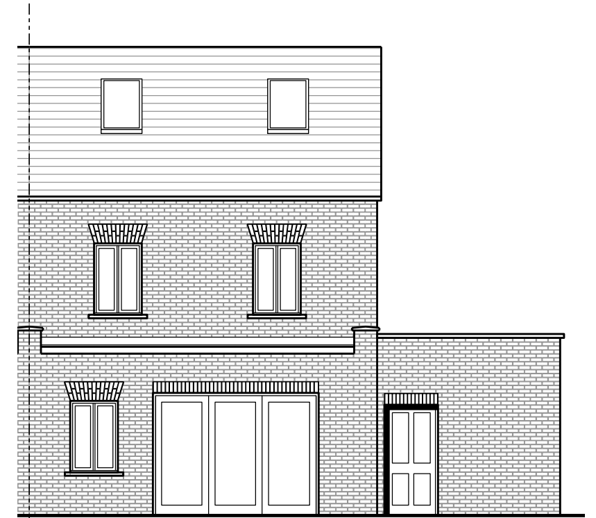
Rear Elevation House Type C1
