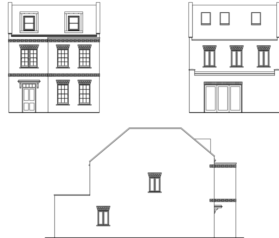
Figure 4.1: Elevations demonstrating proportions of glazing at front, rear and side of typical new-build houses (House type E1 used as example)
