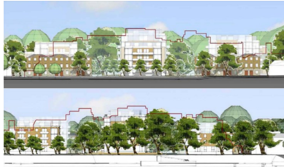
Figure 21: Proposed elevations from the River Thames (top) and Broom Road (bottom). The red line indicates the current massing of Teddington Studios within these views, indicating that the proposed development falls within the site's existing massing boundary.
