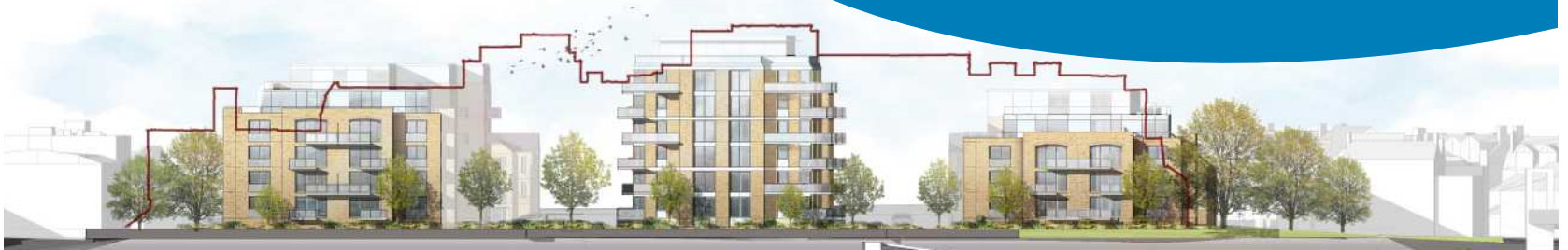
Elevation to River Thames showing proposals with existing building line in red
