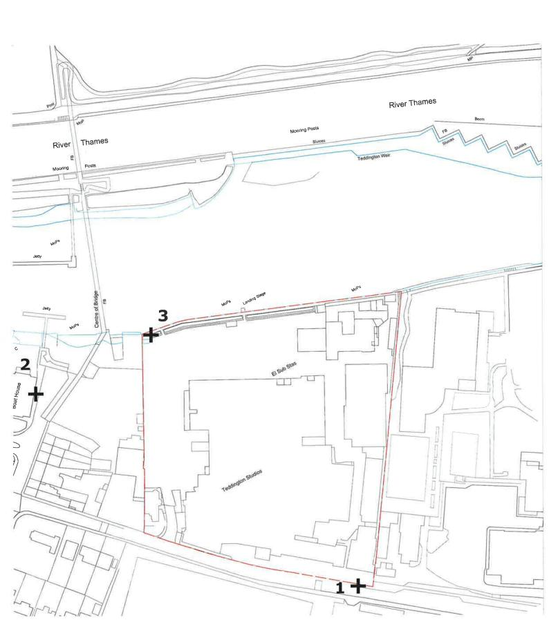
Figure 8.1: Site location and noise measurement positions
