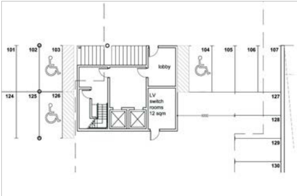
10% of parking spaces are reserved alongside lifts for blue badge holders. All stairs are hobbled, as is the lift lobby. Cycles are secure by virtue of the overall car parks securely and are CCTV monitored. Screen walls are low level and all areas brightly lit and wall and floor surfaces decorated or demarcated.
