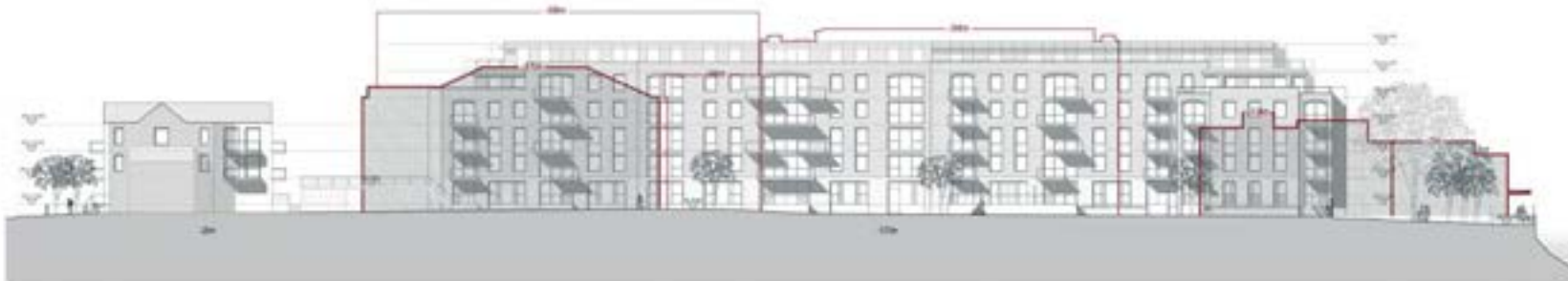
Elevation 4-4' (figured dimensions are the distance an existing or proposed plane is away from its relevant boundary)
