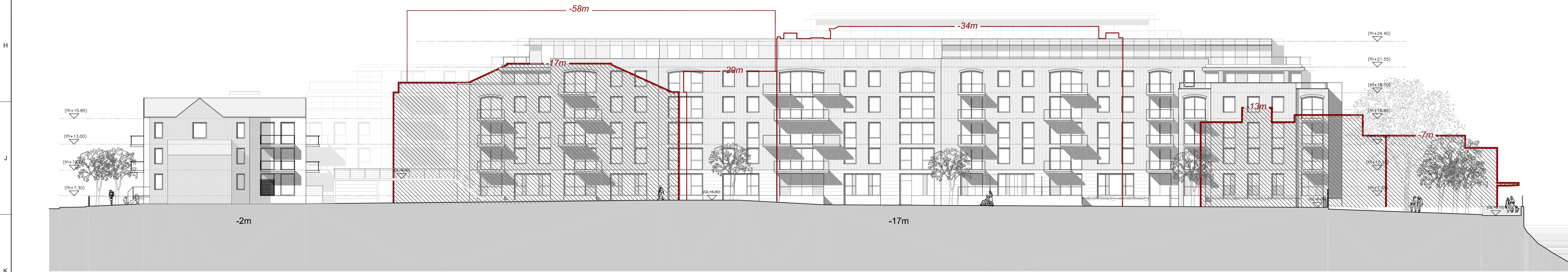
Elevation 4-4' (figured dimensions are the distance an existing or proposed plane is away from its relevant boundary)
