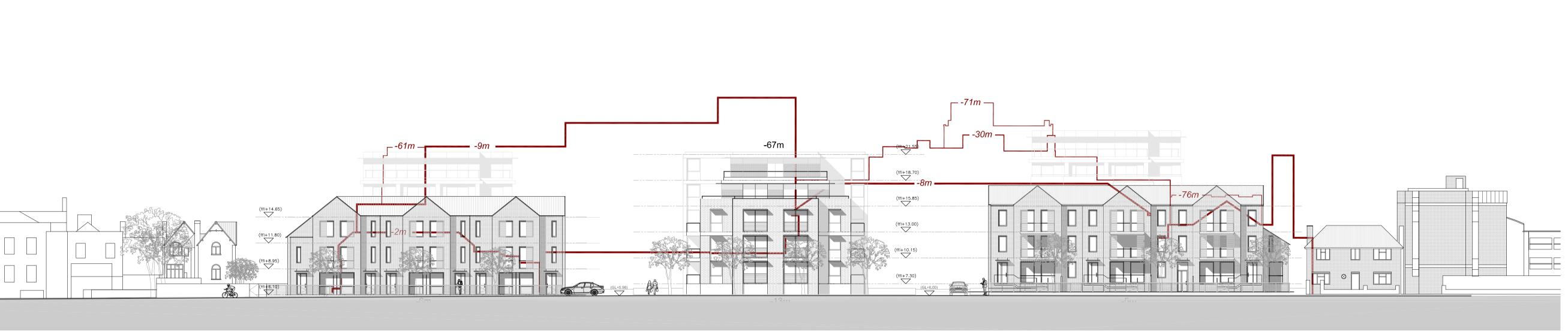
Elevation 1-1' (figured dimensions are the distance an existing or proposed plane is away from its relevant boundary)
