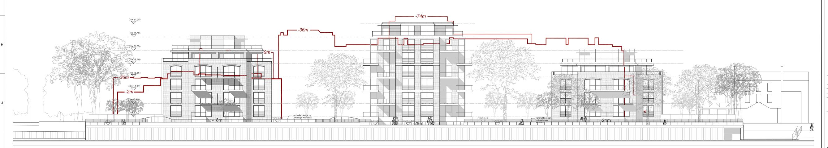
Elevation 2-2' (figured dimensions are the distance an existing or proposed plane is away from its relevant boundary)
