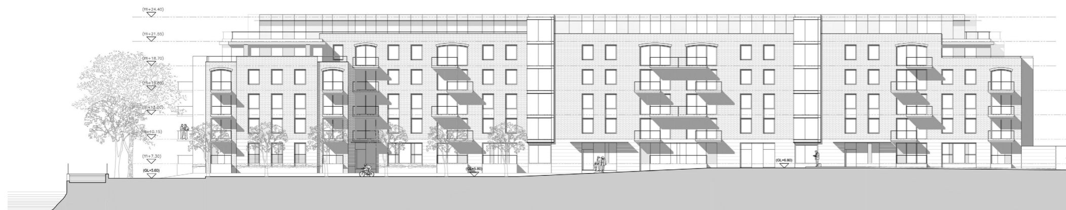
Above: A & C step down at their northern and southern ends.
