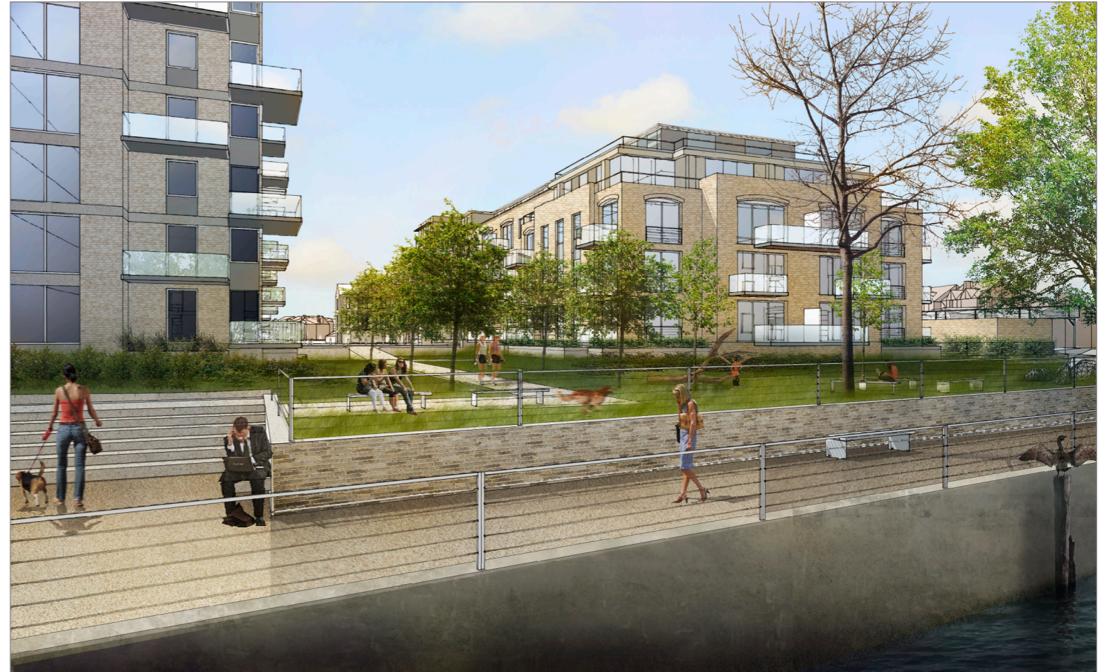
Above: the parkland setting. The front handrail is at the very water edge, while the wall and steps beyond rework the flood defence walls that are perpetuated under the proposal. This involves delicate calculation and even the area beneath the steps is utilised to perpetuate flood risk criteria defences - 70% of units will be dual aspect and none of the single aspect residences are north facing.
