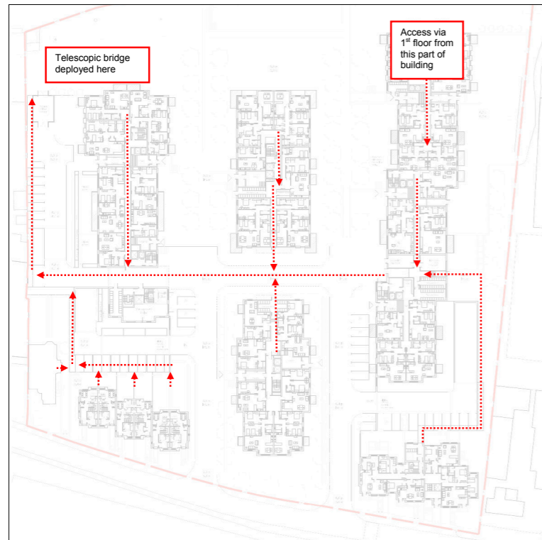
Figure 2 Access/Egress route within the site
