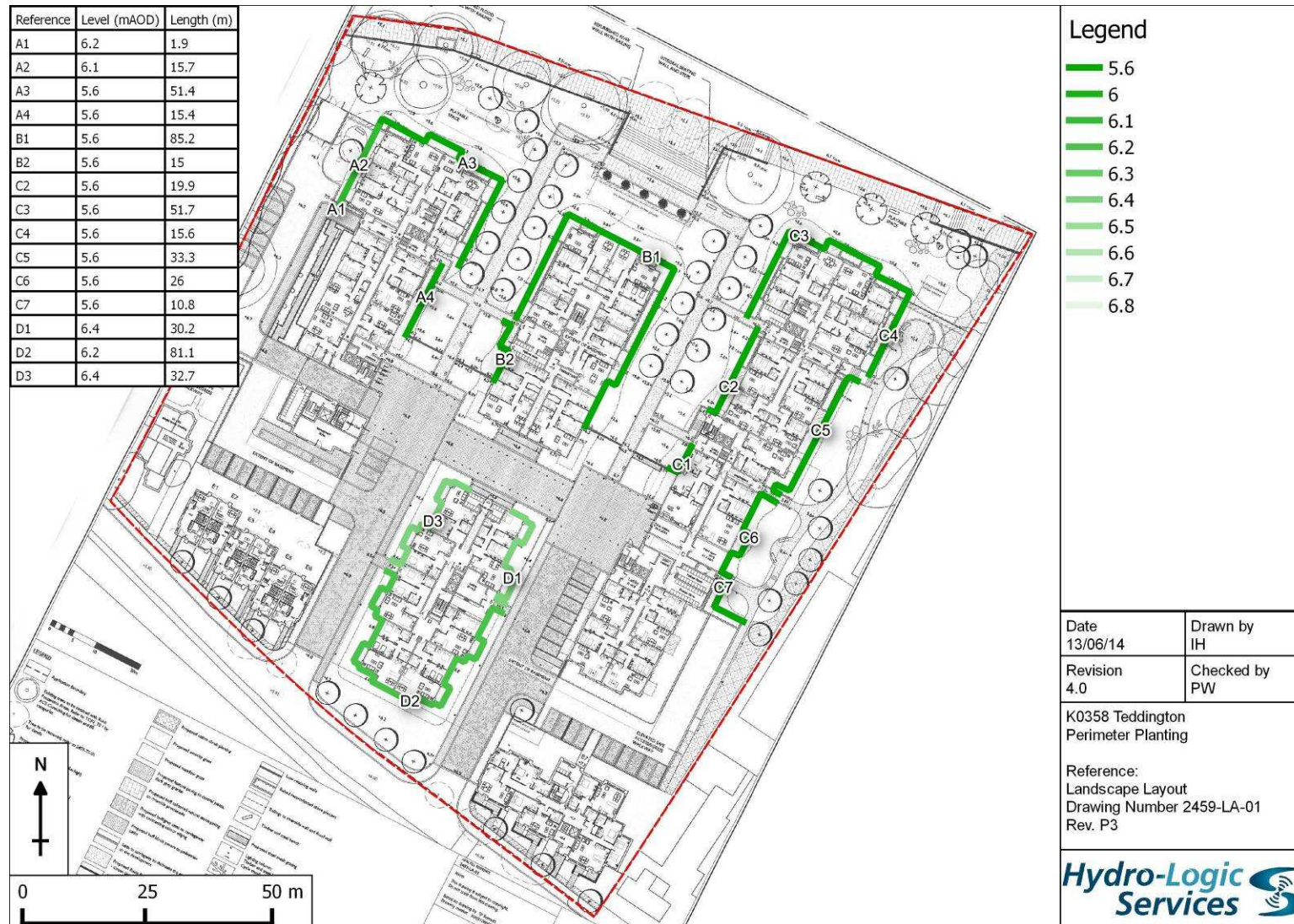
Figure 4-20 Soil embankments around main buildings
