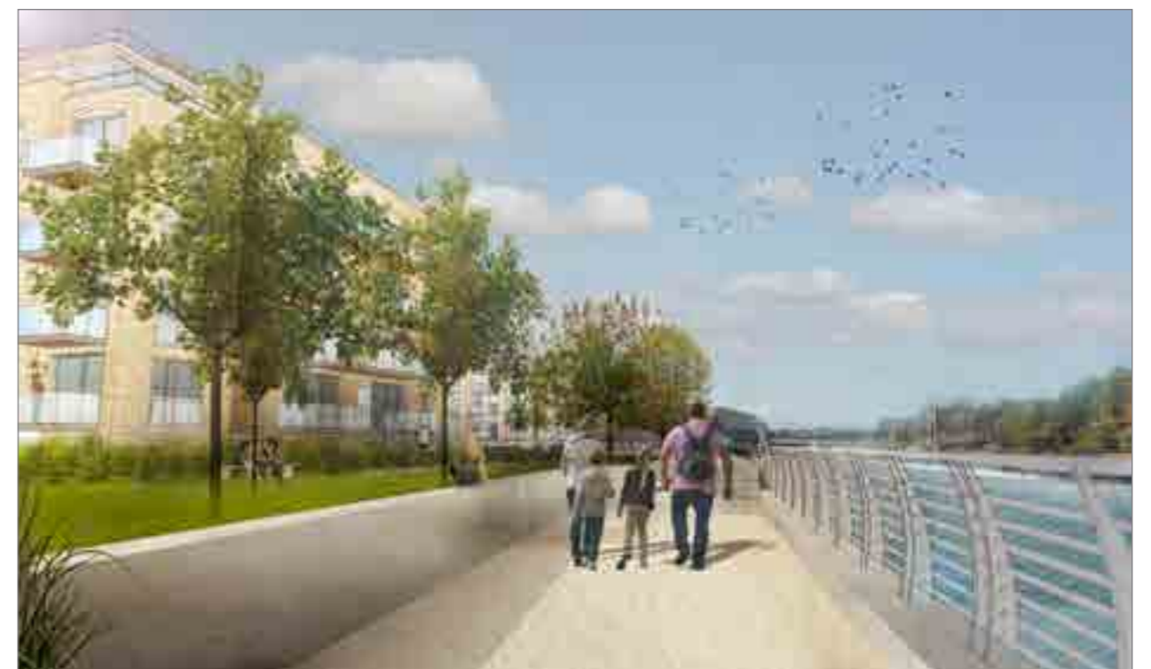
Below: the parkland riverside setting and opposite the central higher piazza maintaining a safe strategy in flood management terms and beyond the lower level which could hold up to 1.0m or so of flood water, still well below the 7.3 ffr of the apartments.
