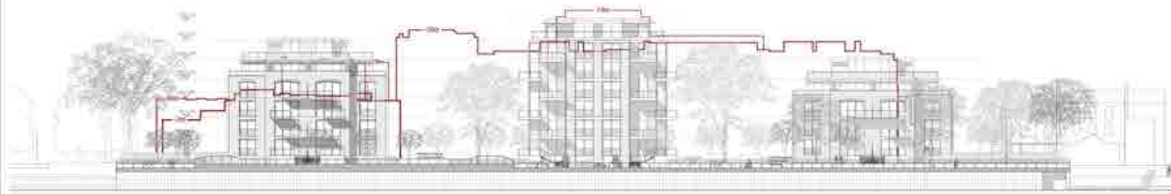
Elevation 2-2' (figured dimensions are the distance an existing or proposed plane is away from its relevant boundary)
