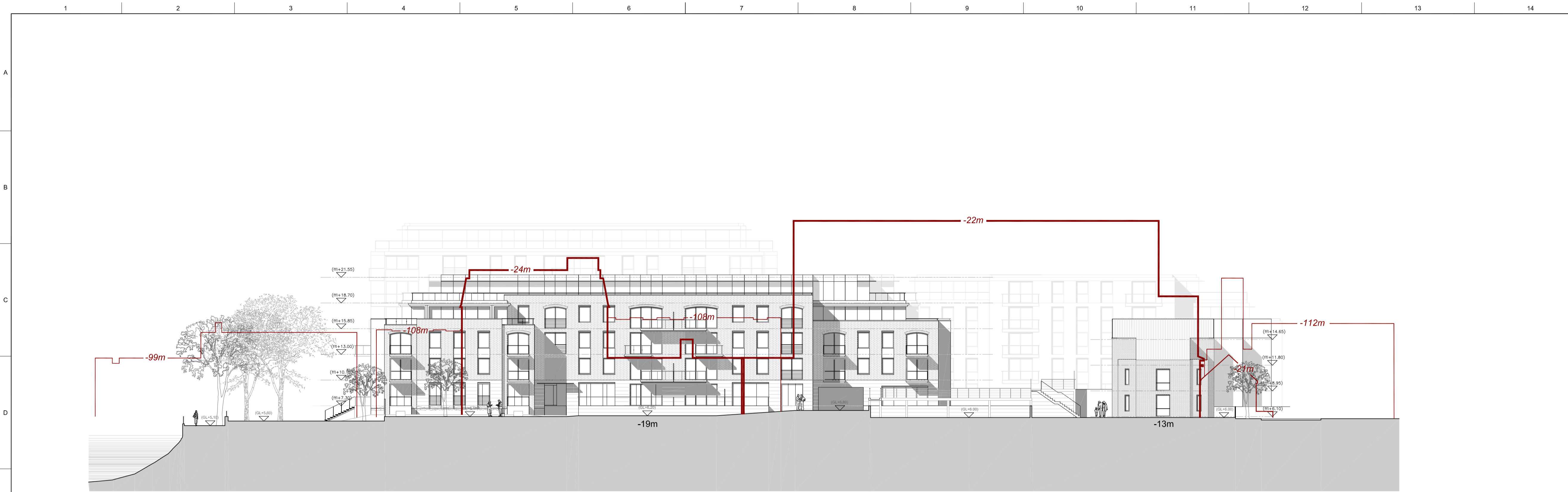
Elevation 3-3' (figured dimensions are the distance an existing or proposed plane is away from its relevant boundary)
