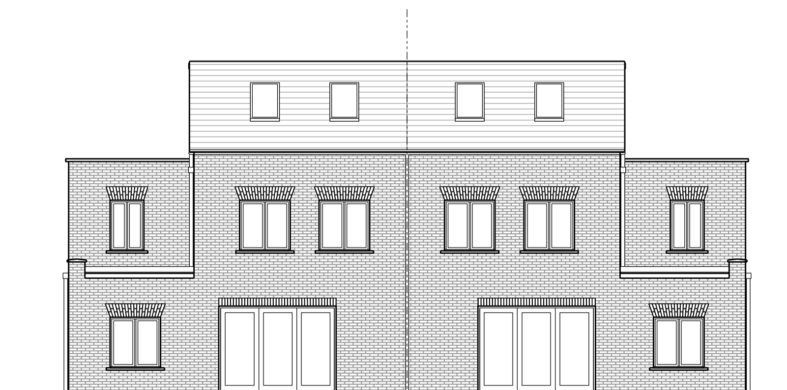
06 Rear Elevation BKH06_P_207 SCALE 1:100
