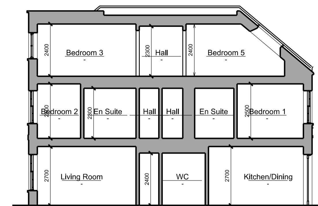
07 Long Section BKH06_P_207 SCALE 1:100
