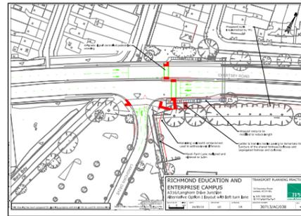
DIAGRAM 6.4.2 DETAILED ACCESS PLAN - JUNCTION OF A316 (AC/038)
