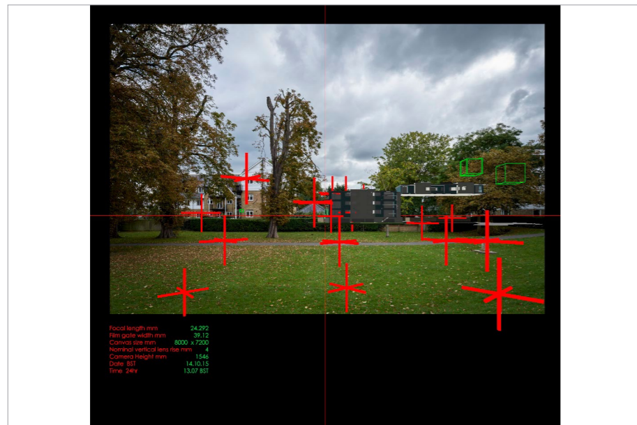
01.7 Screen grab of wireline model matched to photograph (grey block indicates terrain model)
