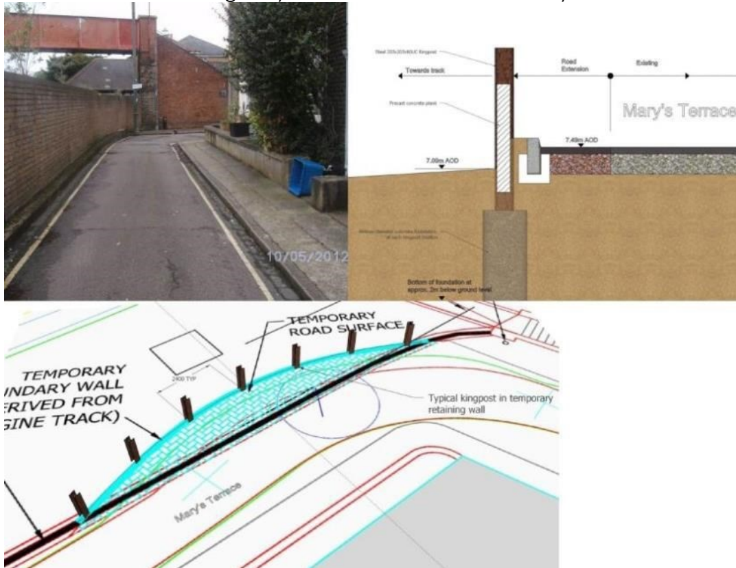
Figure 11 Road widening at the junction with Beauchamp Road to allow fire engine access to Mary's Terrace
