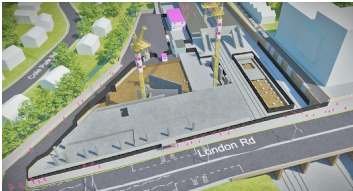
Figure 20 Concrete Frame: pile caps to island
