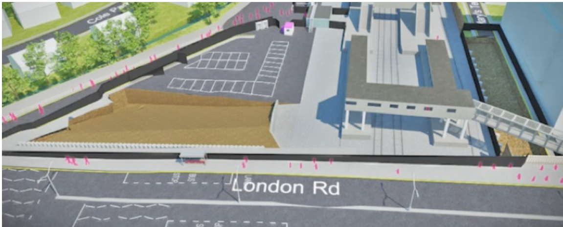
Figure 15: Reduced Dig and Demolition of retaining walls
