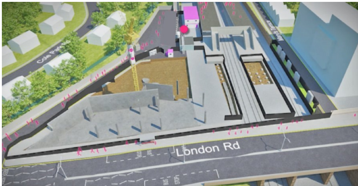
Figure 18 Block A Frame and Island Pile caps
