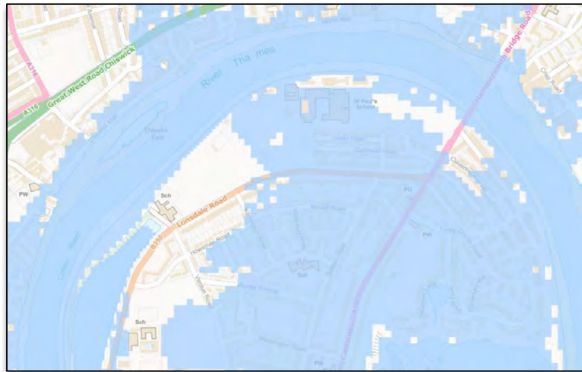
Figure 8: Maximum extent of flooding from reservoir failure (Source EA Online)
