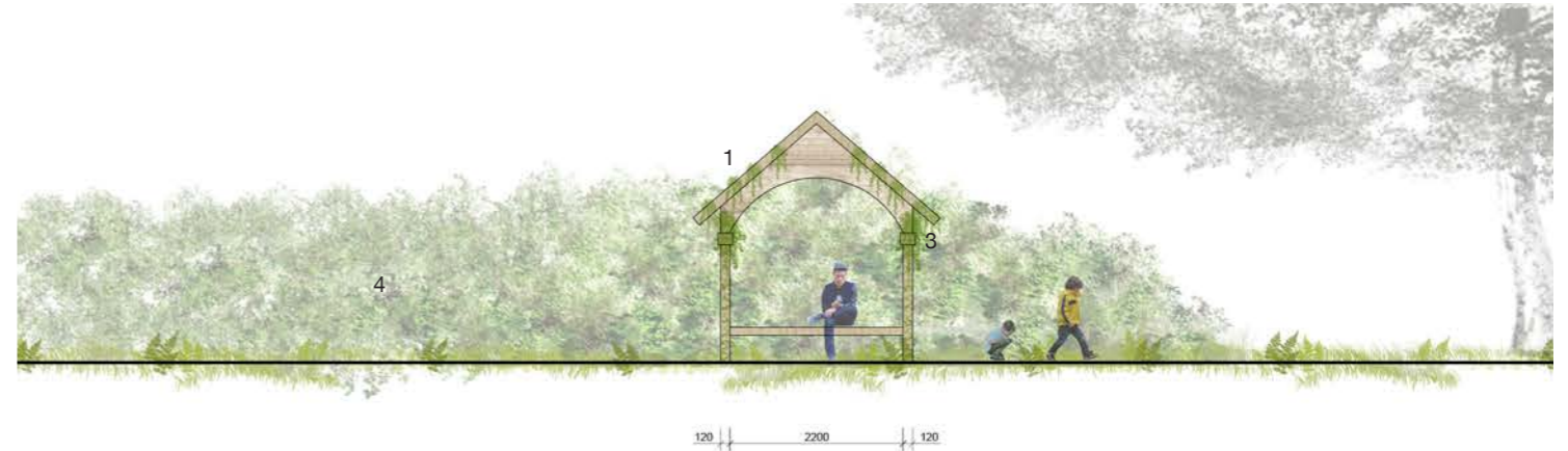
Ice House Seat: Timber frame structure containing a bench, taking reference from the 1752 plan. Ref. 581_PL_L_18
