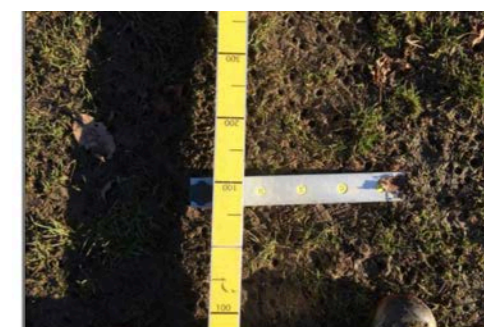
Plate 14: Undulation > 25mm depth – centre circle
