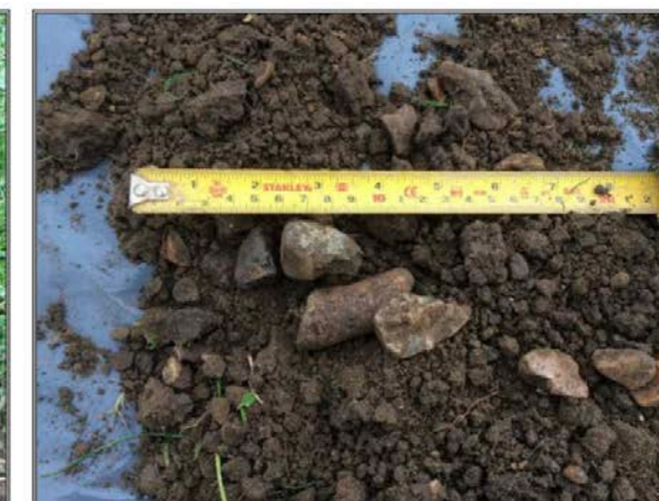
Plate 12: Subangular and subrounded, small to medium sized stones within Profile 1 Topsoil
