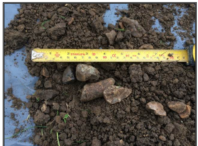
Plate 8: Subangular and subrounded, small to medium sized stones within Profile 1 Topsoil
