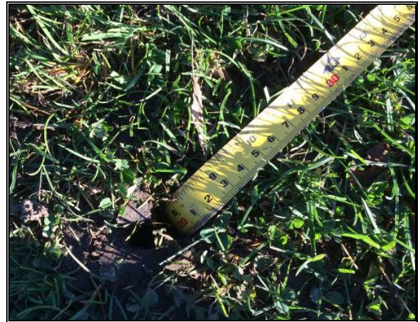
Plate 19: Measured depth of vert-drain hole 210mm
