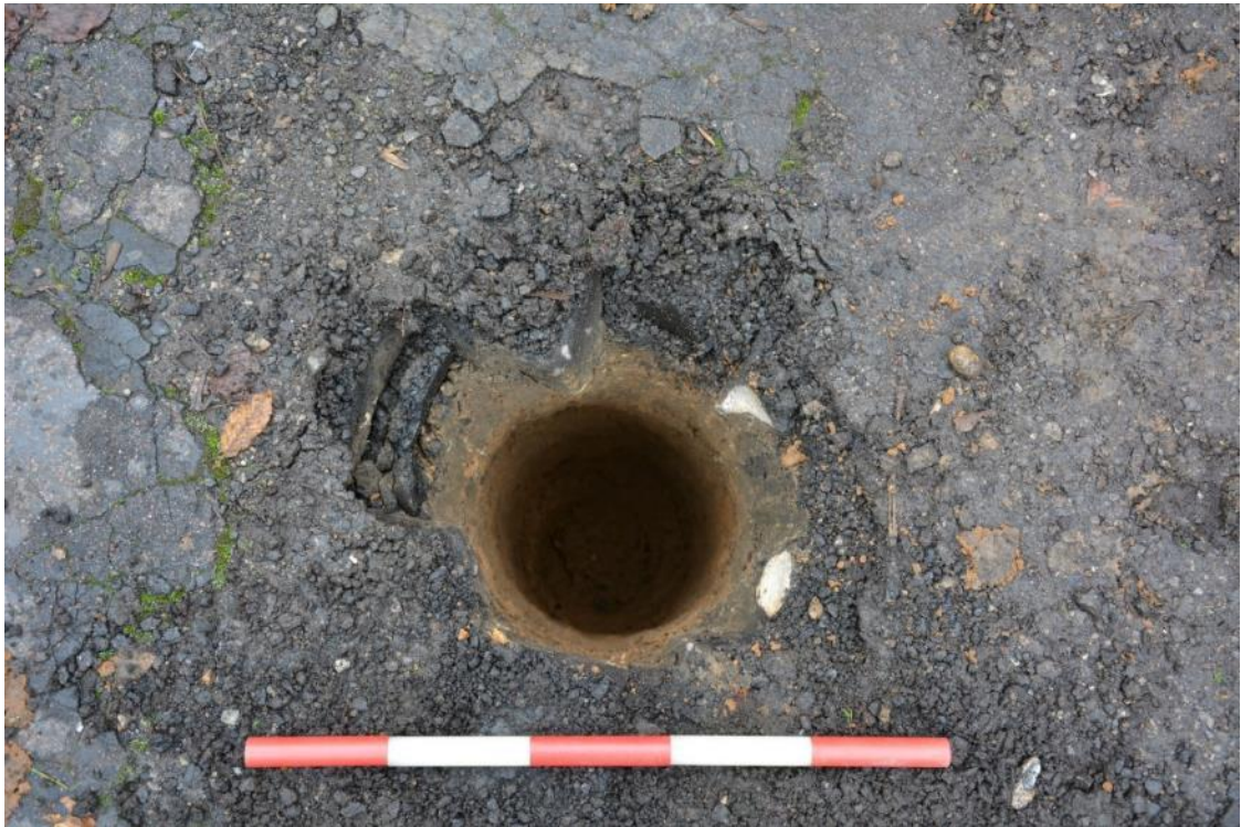
Figure 20 - Borehole 1, upper metre prior to window sampling.
