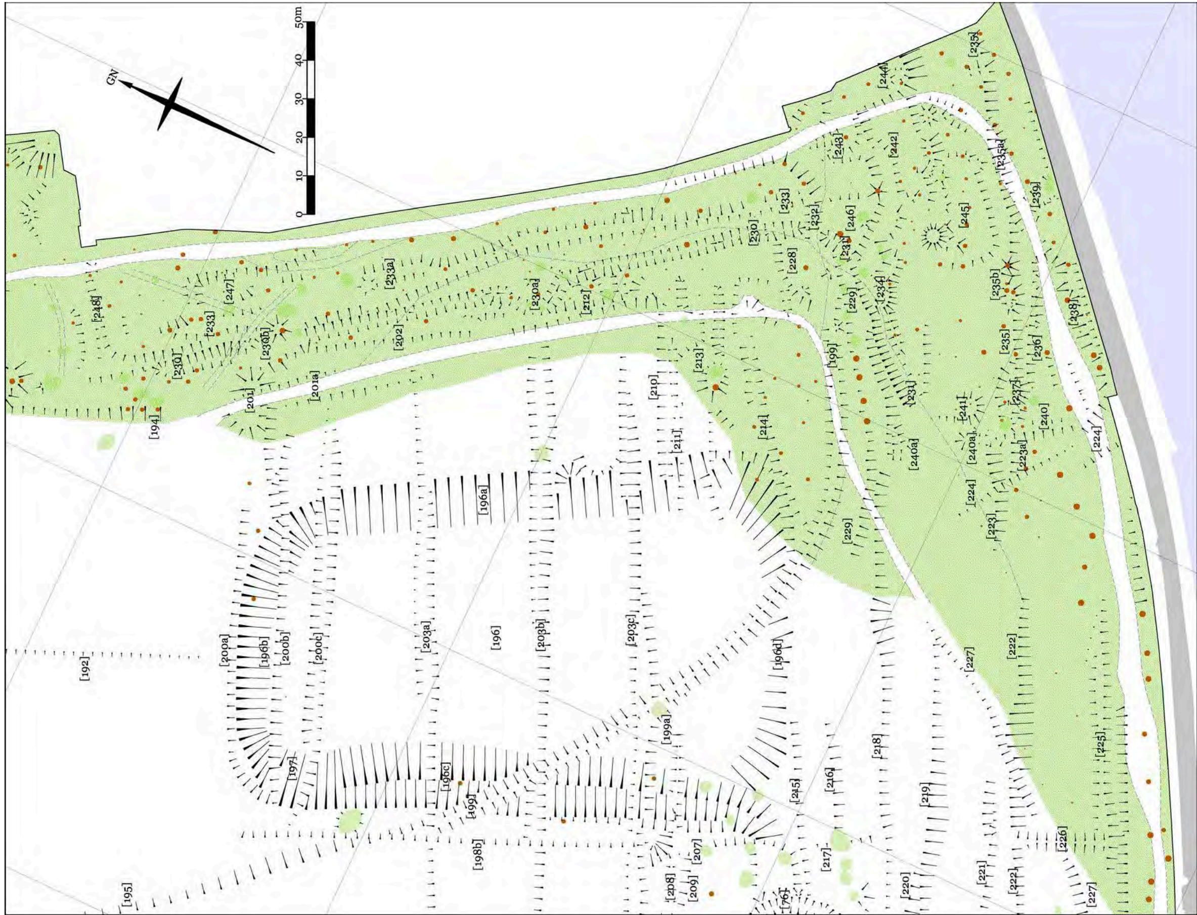
Figure 42 – Earthwork survey in the south of East Meadow and Little Marble Hill 1:1000@A3 (background Greenhatch Group 2015 © Historic England)
