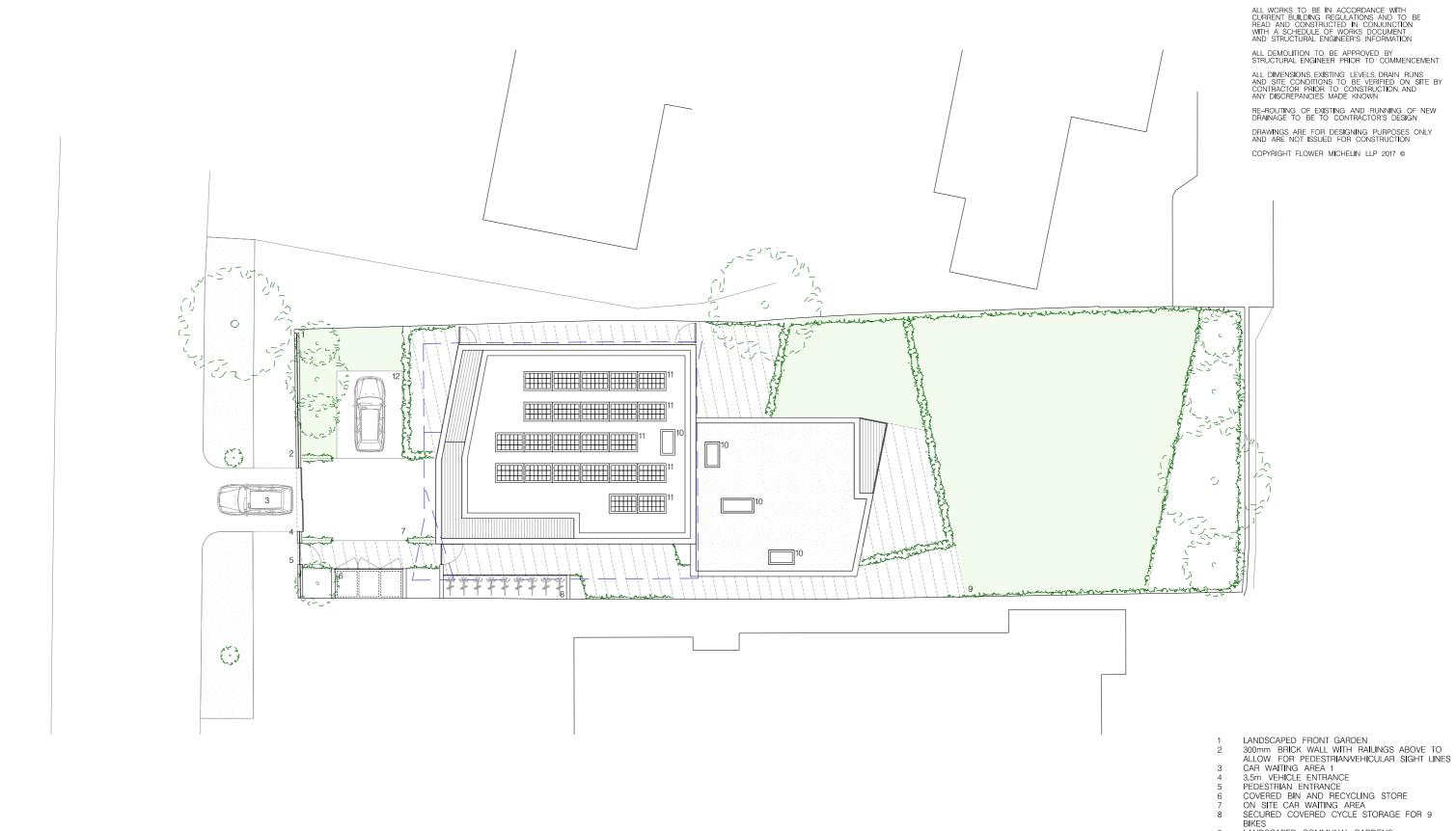
Rev. A Drawing revised to show PV panels to roof
