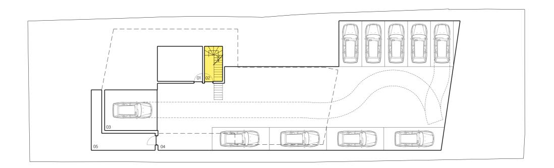
01 PLANT ROOM 02 STAIR TO ENTRANCE HALL 03 CAR LIFT 04 CAR PARKING SPACE (FOR 09 CARS) 05 CAR LIFT MOTOR ROOM
