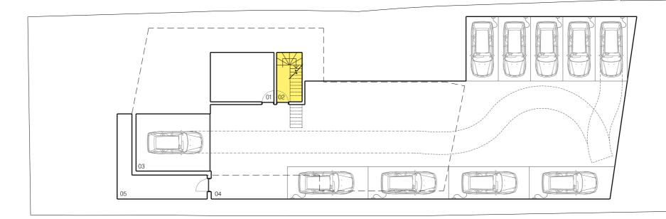
01 PLANT ROOM 02 STAIR TO ENTRANCE HALL 03 CAR LIFT 04 CAR PARKING SPACE WITH EV CHARGING POINTS (FOR 09 CARS) 05 CAR LIFT MOTOR ROOM
