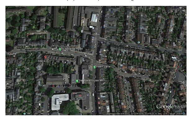
3.4 A Norsonic 118 type 1 sound level meter was deployed at MP1 for the duration of approximately 24 hours. The meter was calibrated at the start and end of measurements and no significant measurement drift was noted. The meter was set to measure over 15 minute time periods and record the parameters  $L_{Aeq}$ ,  $L_{Amax}$  and  $L_{A90}$ .
