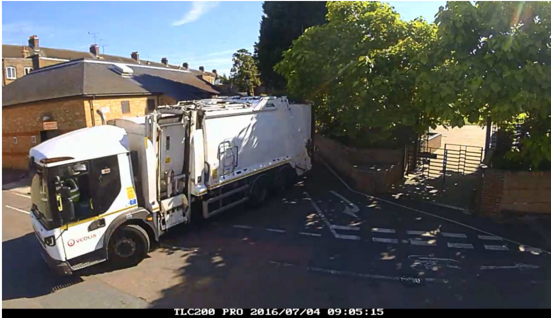
Figure 3.10 Service Road – Large Refuse Overrunning Kerb
