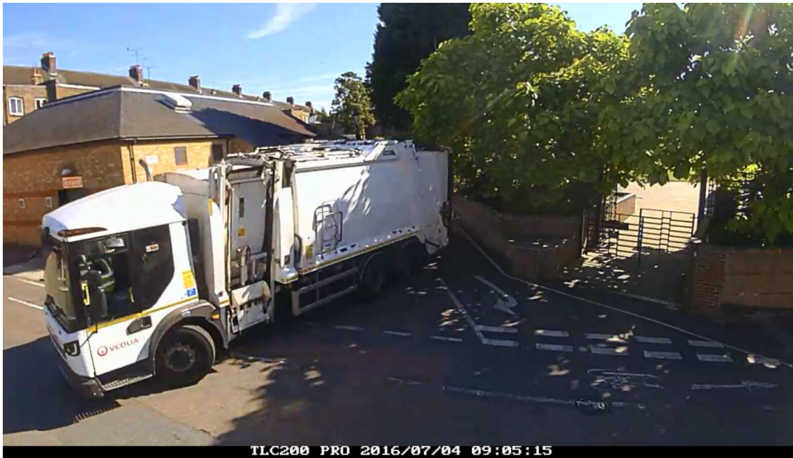
Figure 3.10 Service Road – Large Refuse Overrunning Kerb
