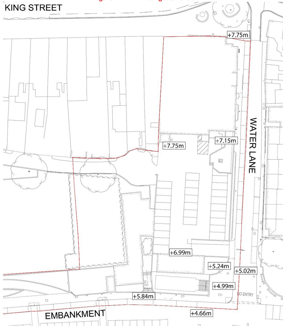
Figure 1. Existing Site Levels
