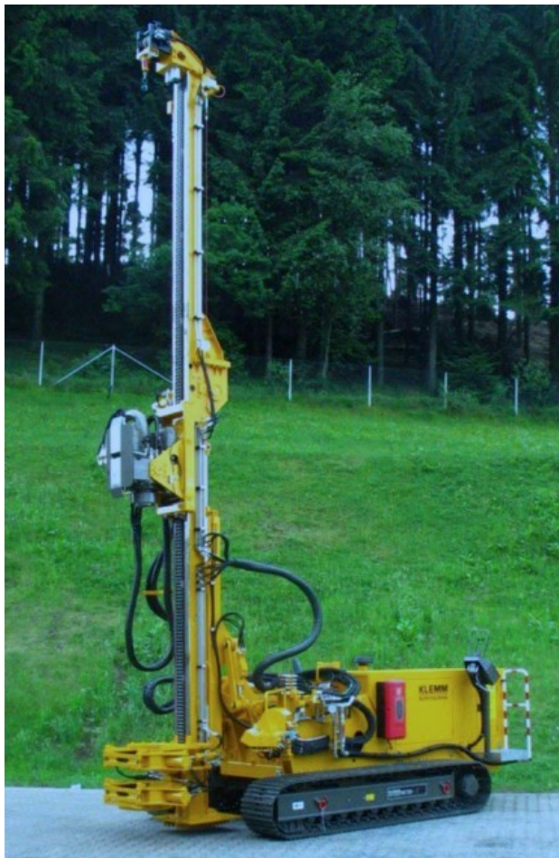
Figure 22; Klemm KR 709 Restricted Height Type Piling Rig
