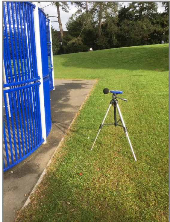
Figure 2 – Source noise Measurement positions and MUGA Backboard
