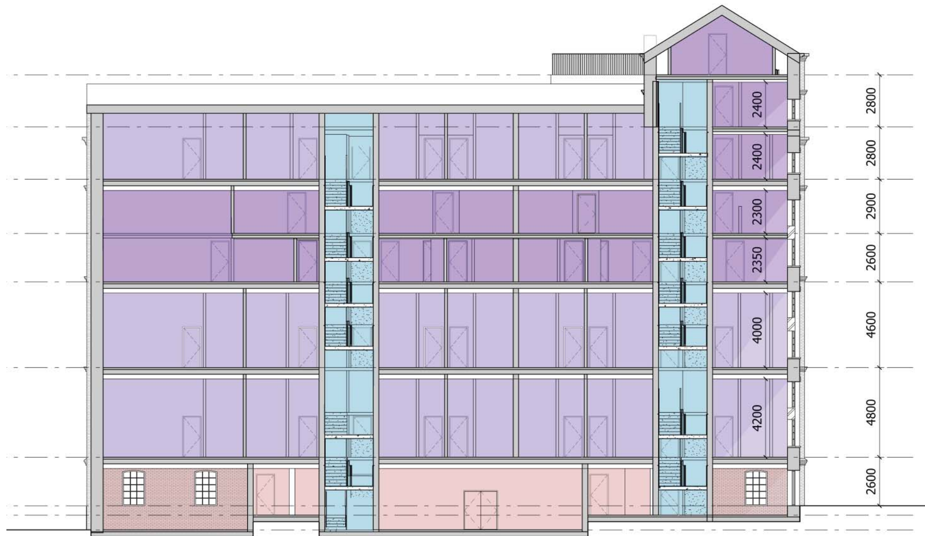
Proposed long section through Maltings building
