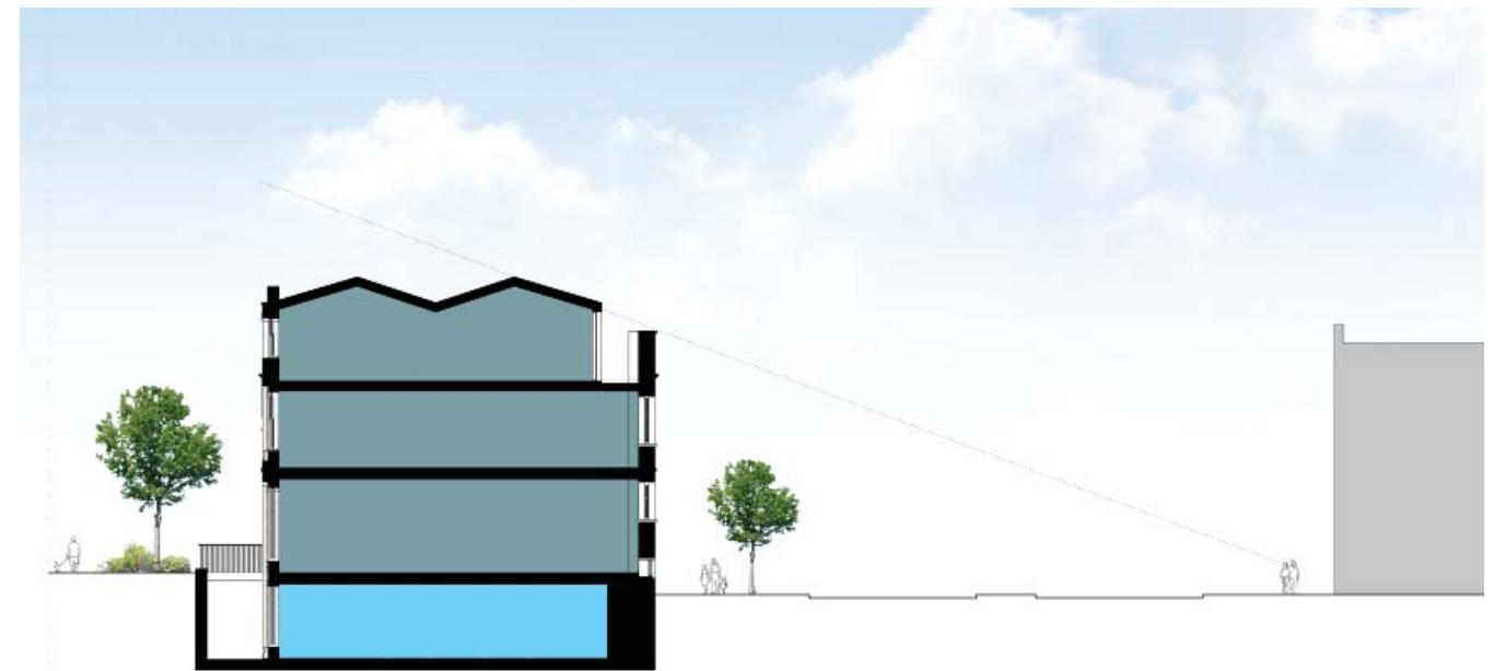
Proposed section through Bottling Building roof - line showing visual impact of roof above parapet level
