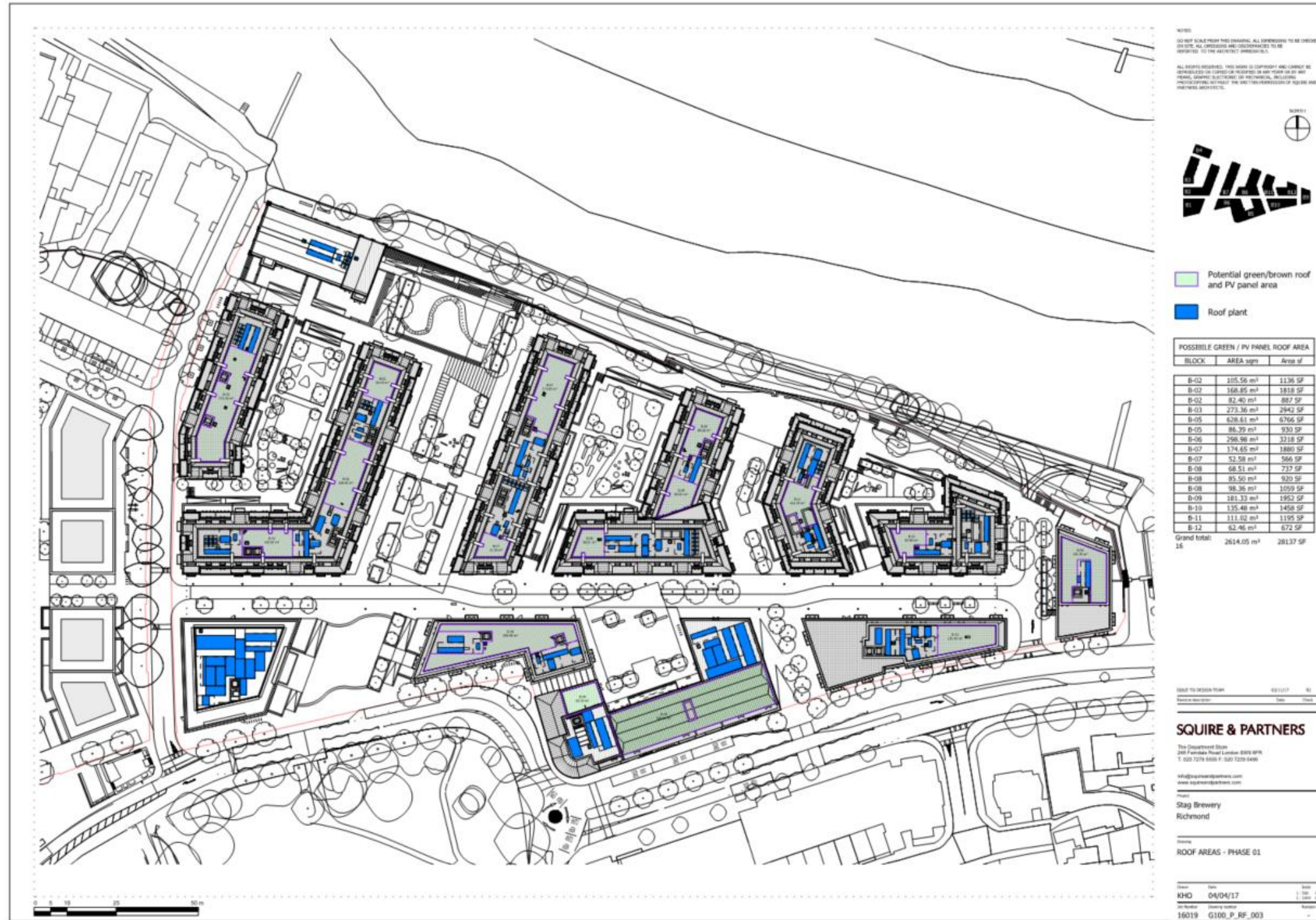
Figure D1: Roof Layout for PV/Green/Brown Roof on Development Area 1 (shown in Green)
