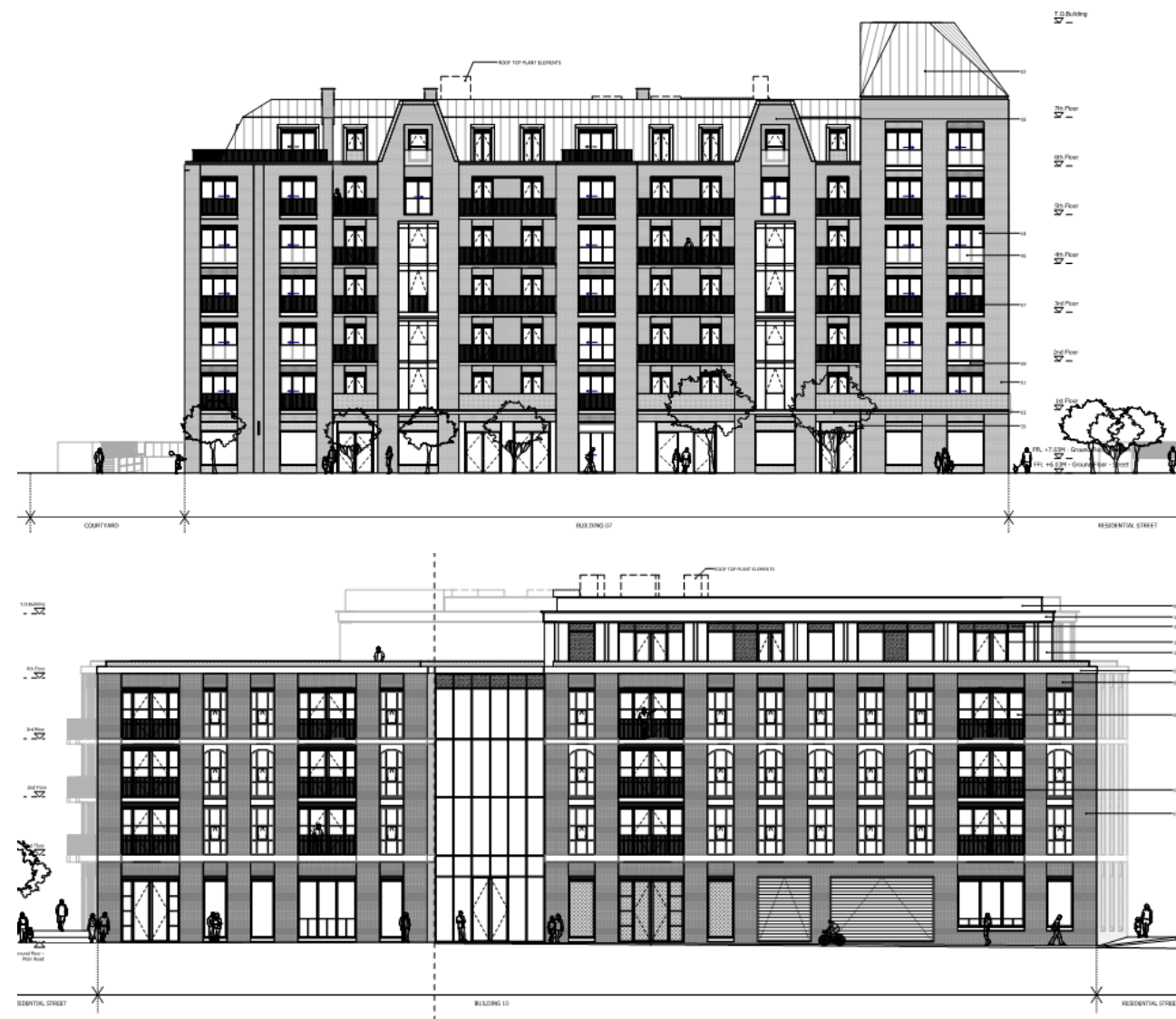
Figure 4.21: Typical Window Openings of Block 08 and 10 South Elevation (Source: Squire and Partners).
