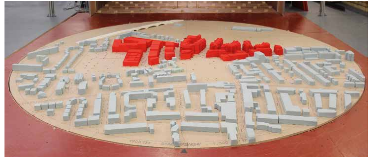
Configuration 2: The Development with existing surrounding buildings - View in the Wind Tunnel (from the south)
