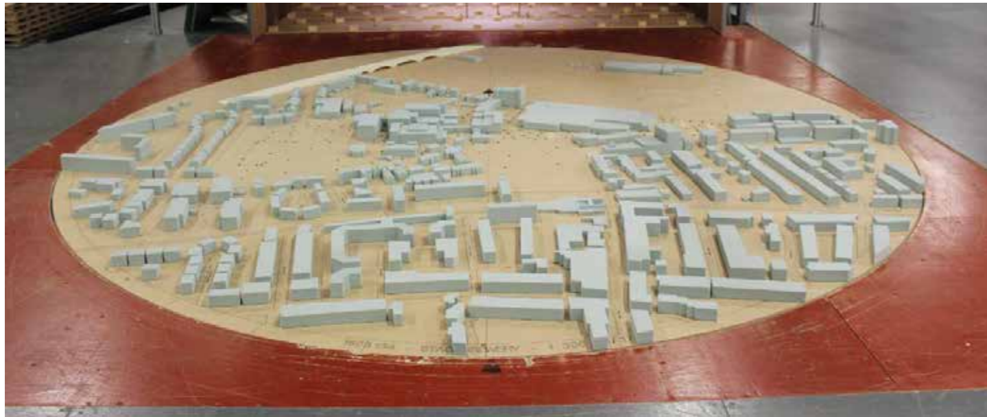
Configuration 1: The existing Site with existing surrounding buildings - View in the Wind Tunnel (from the south)
