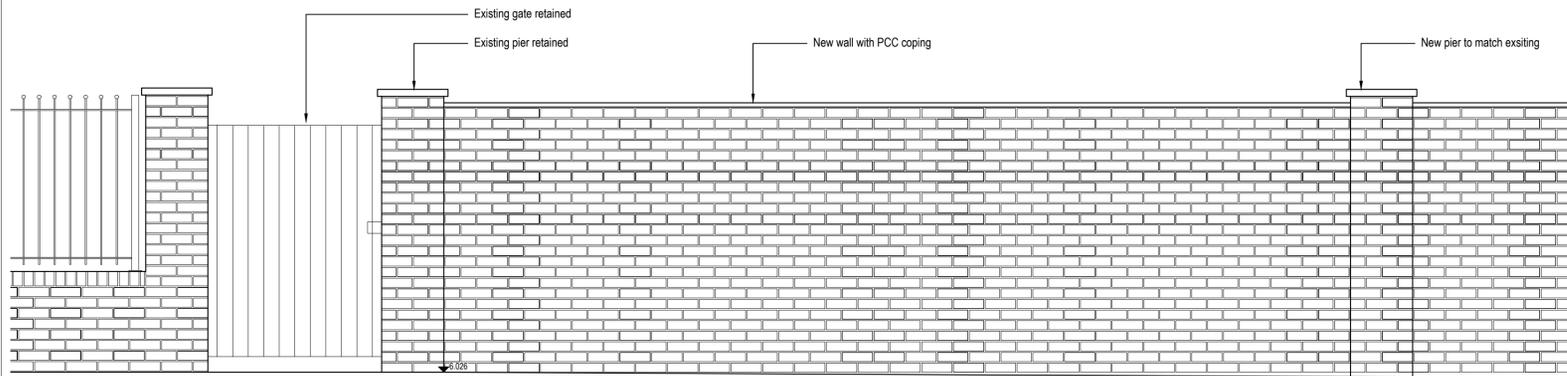
**E** PROPOSED WALL ELEVATION DETAIL
