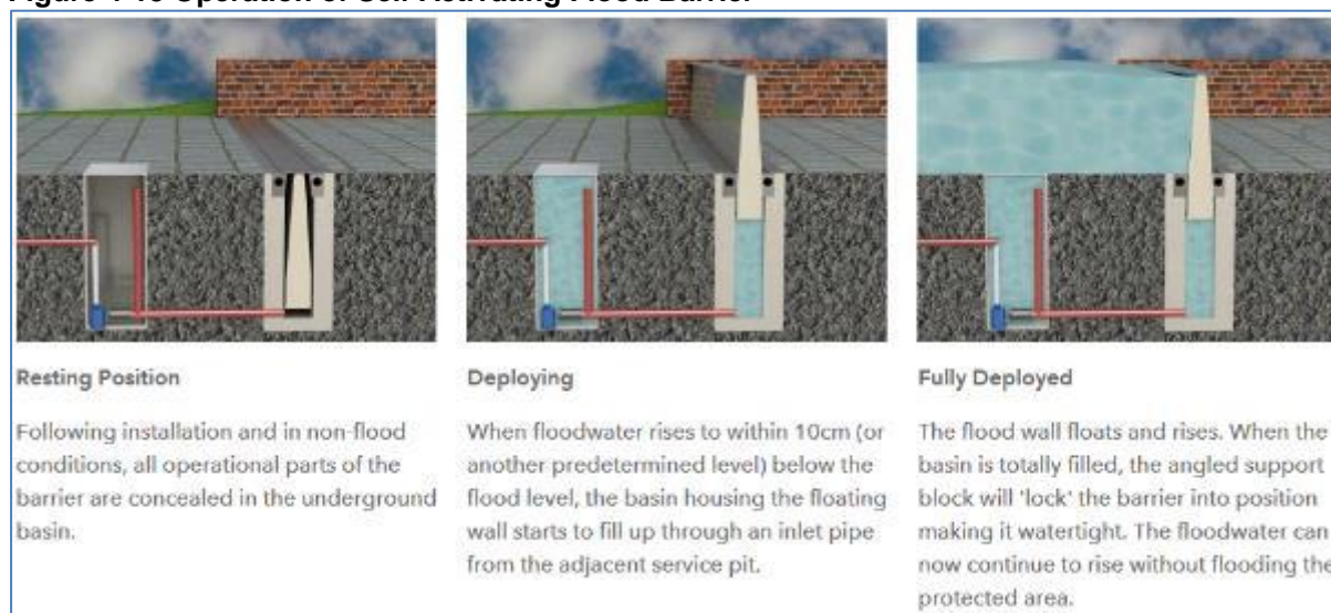
Figure 4-15 Operation of Self Activating Flood Barrier
