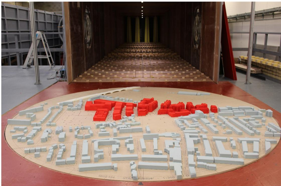
**Figure 2: Image of the Development with existing surrounding buildings. (View in the wind tunnel from south)**
