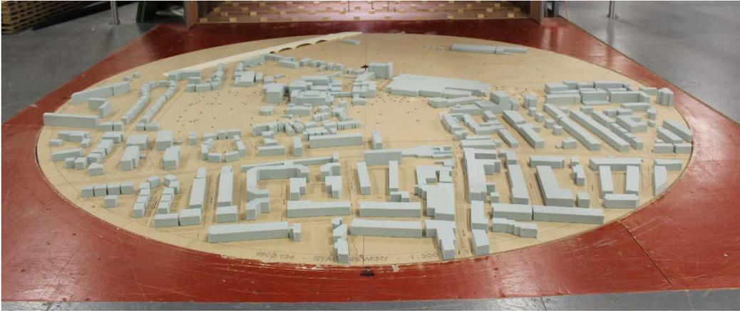
**Figure 11: The Existing Site with existing surrounding buildings (Configuration 1) – View in the Wind Tunnel (from the south)**
