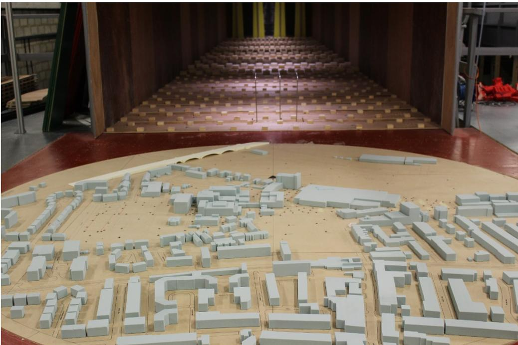
**Figure 12: The Existing Site with existing surrounding buildings (Configuration 1) – View in the Wind Tunnel (from the south)**
