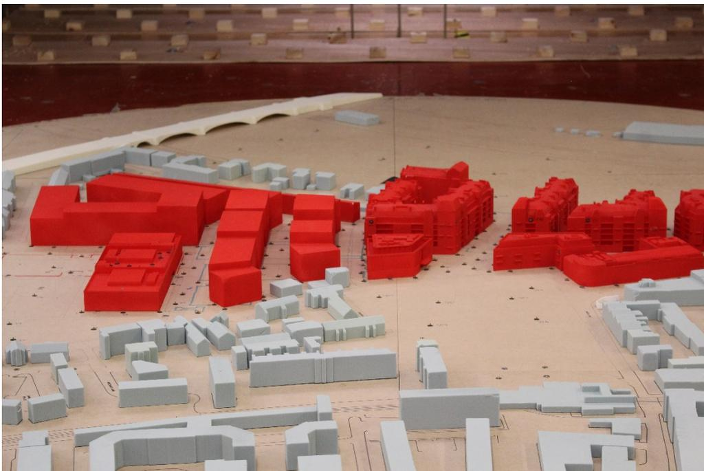
**Figure 14: The Development with existing surrounding buildings (Configuration 2) - View in the Wind Tunnel (from the south)**
