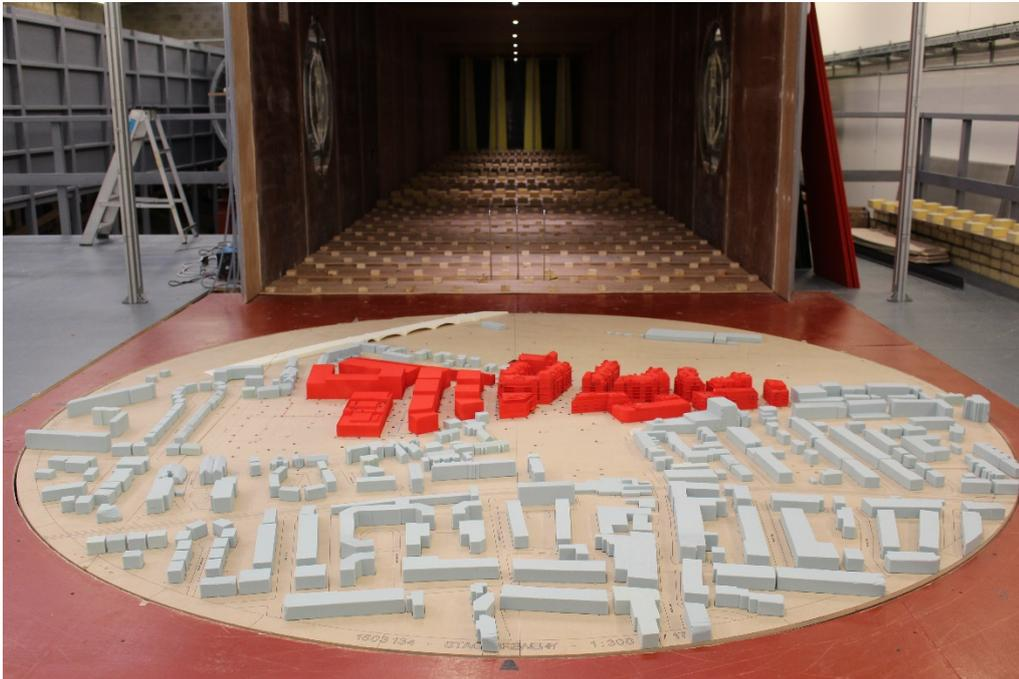
**Figure 13: The Development with existing surrounding buildings (Configuration 2) - View in the Wind Tunnel (from the south)**
