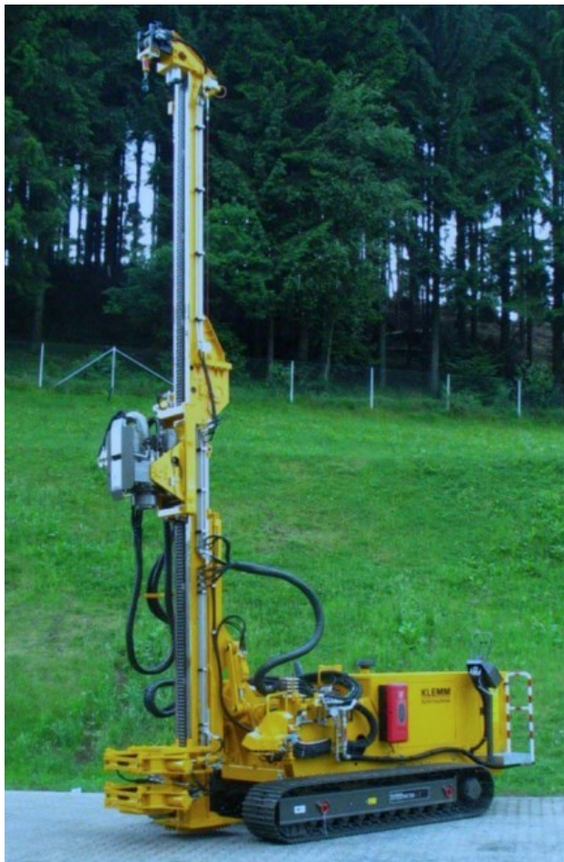
Figure 22; Klemm KR 709 Restricted Height Type Piling Rig
