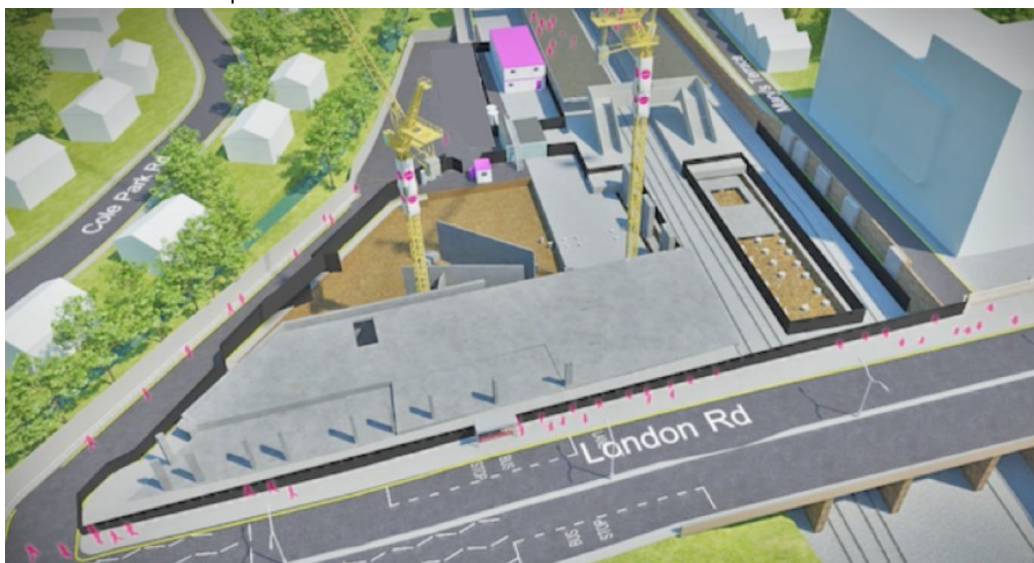
Figure 23: Concrete Frame: Pile Caps to Island
