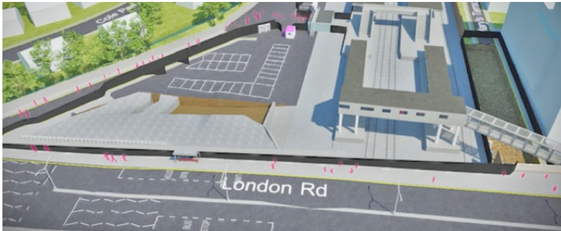
Figure 16: Contiguous Piling and Mary's Terrace Road Closure
