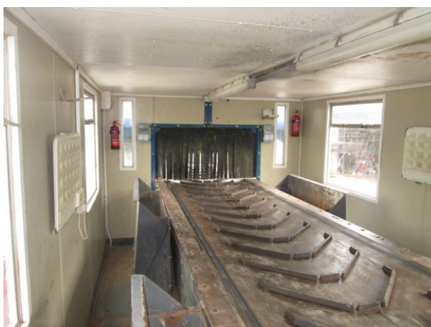
Figure 18: conveyor belt in enclosed area to sort ACMs
