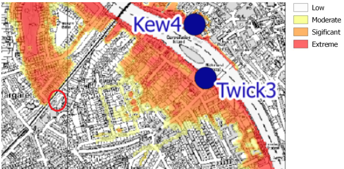
Figure 2.2 Flood Hazard due to a Breach of the Defences
