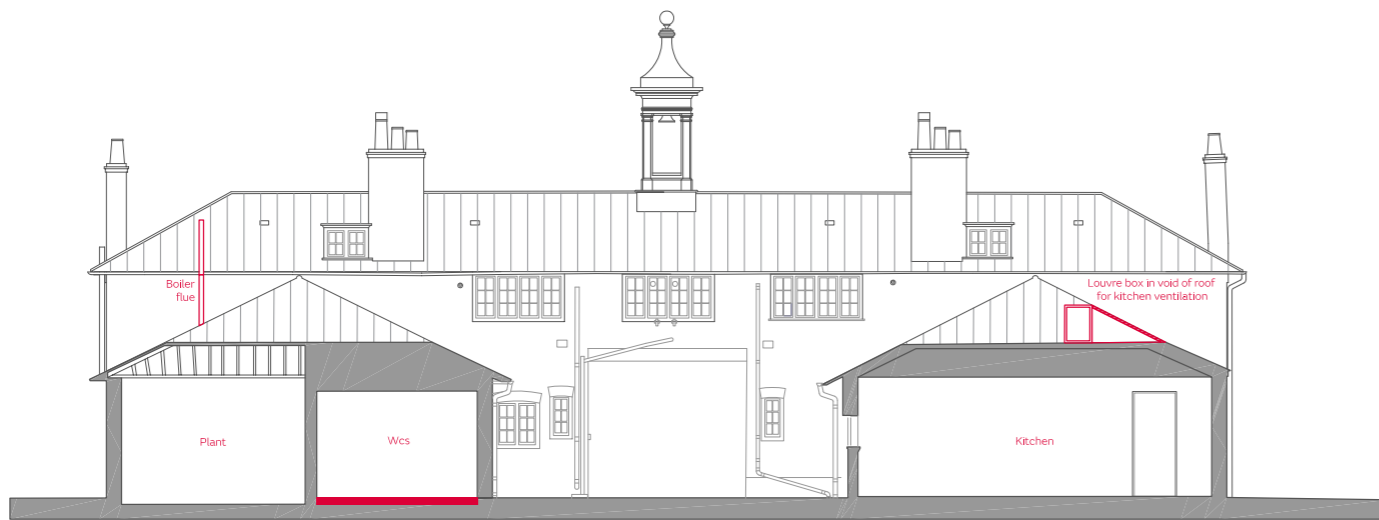
Section through ancillary wings to Stable Block
