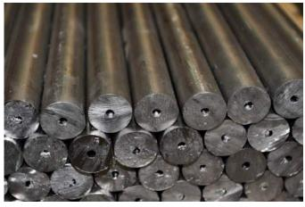
Sash Weights; where required assume all new sash weights should be round lead weights from 'The Leadweight Company.' Weight diameters from 25 - 50 mm are available, size to suit sash lining. The weights should be fitted with eyelet fixings.
