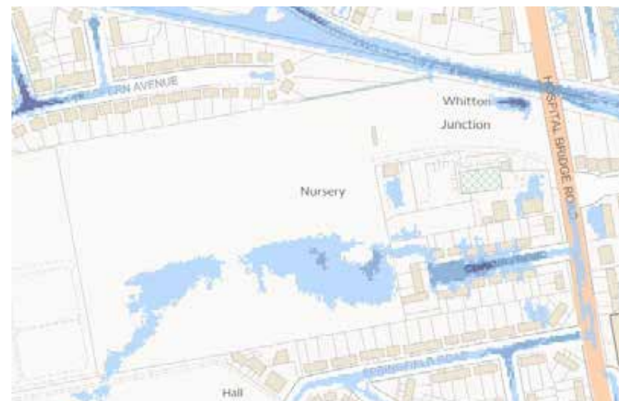
Surface Water Flooding (Data taken from EA Mapping)
